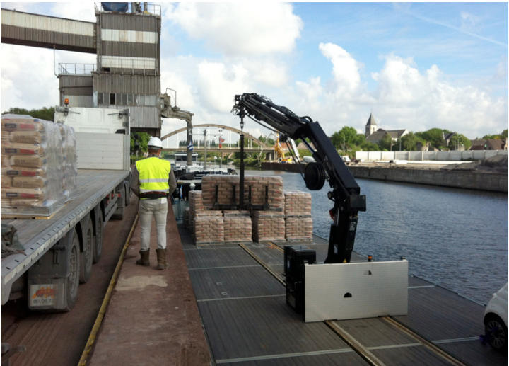
Traditional inland vessels are not suitable for transhipment of palletised goods. Thanks to the crane on the boat, there is no need for large infrastructure on the quay.
